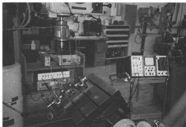
Fig. 8 Experimental setup for drill life tests.
